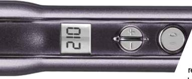
The LCD screen allows to control the selected temperature level. The temperature on the display will flash while the iron is heating up to the selected temperature. When the selected temperature has been reached, the temperature display will stop flashing.
